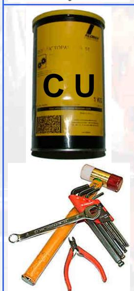
Apply copper grease on the threads of both catalytic converter plugs (easier assembly and disassembly).
