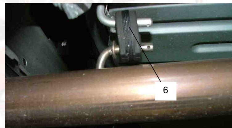
**Nota :** The final tube of exhaust line has to be shorter than the longest point of the car (in accordance to the FIA rule).
